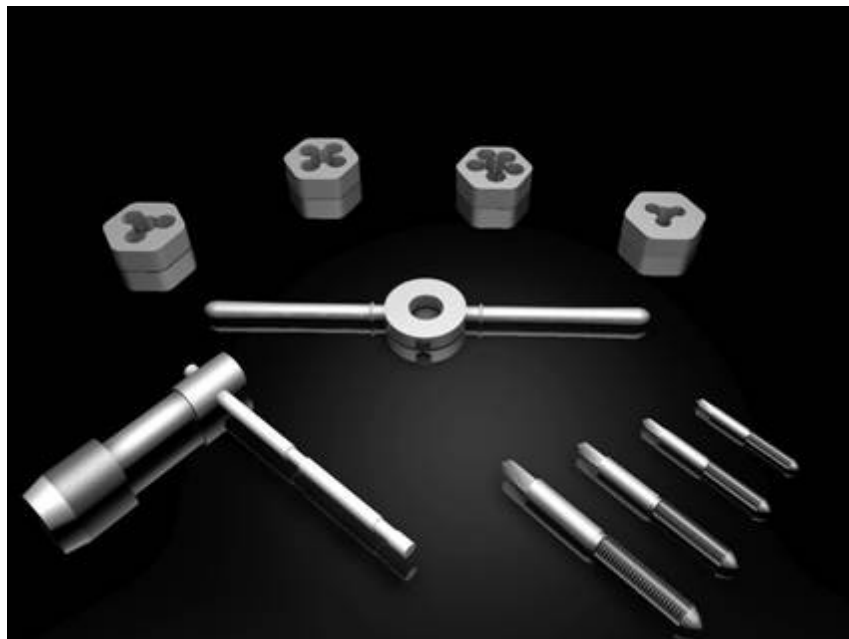
Dies in back row, die wrench in center, tap wrench in lower left, and taps in lower right.
