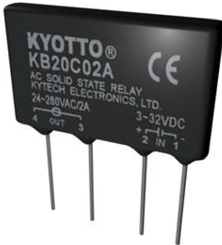
Kyotto Solid State Relay. Control pins are 1 and 2 and require 3–32 volts. Switched output pins are 3 and 4. The maximum rating for these pins is 2 amps at any voltage between 24 and 280 volts AC.
