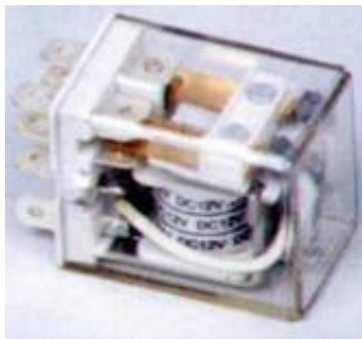
Electromagnetic relay. As a coil creates a magnetic field, it pulls a switch down.
