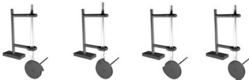
Snail cam and a vertical follower with a roller shoulder bolt at the end that makes contact with the spinning cam.
