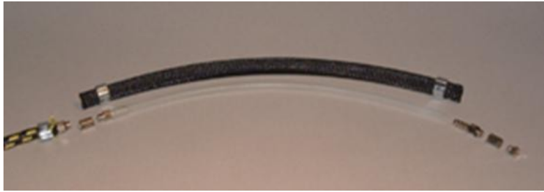
Rubber tubing below polyester sleeving.
