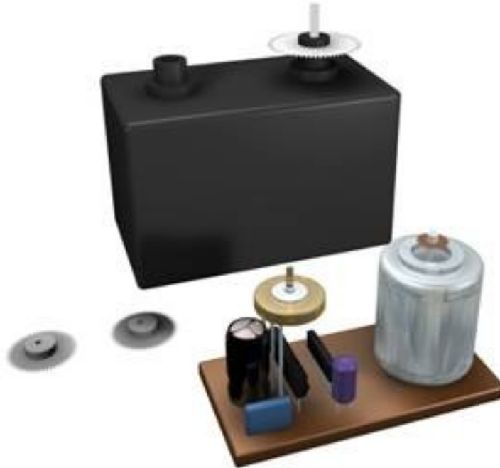
Servo motor deconstructed, showing the potentiometer and gears. The pot is the encoder for the motor.
